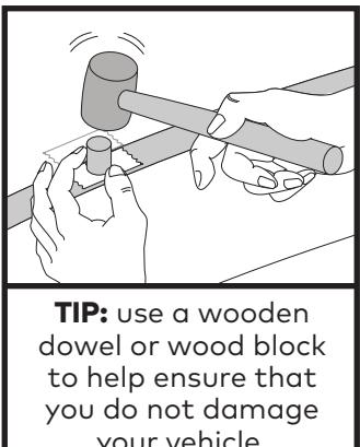
**TIP:** use a wooden dowel or wood block to help ensure that you do not damage your vehicle.
