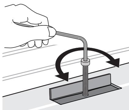
NOTE: Some vehicles have a plug in the threads which must be removed.
