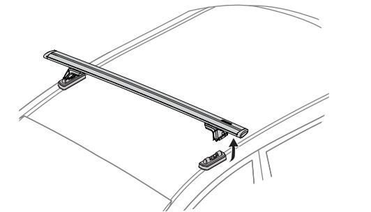
E. While holding the SkyLine or Control Tower above the Landing Pad, fully tighten Landing Pad to 1.5 Nm (13.3 in lb) (use the long end of the wrench as shown). DO NOT OVER TIGHTEN AS DAMAGE TO THE ROOF MAY OCCUR.
