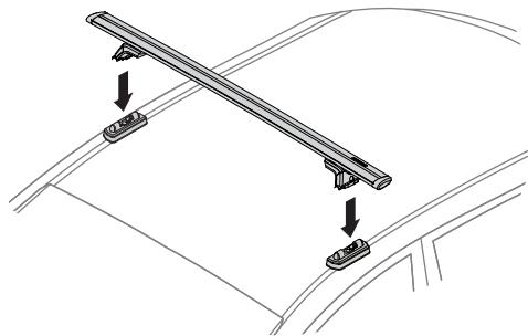
B. Align position of Landing Pads to allow SkyLine or Control Towers to fully close.
