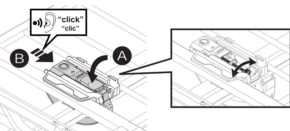
**Adjust strap tension and close the levers.** Strap tension can be adjusted by turning the thumbwheel in both directions. Adjust the strap tension with the thumbwheel so the strap is tight around the crossbar when the lever is closed.
