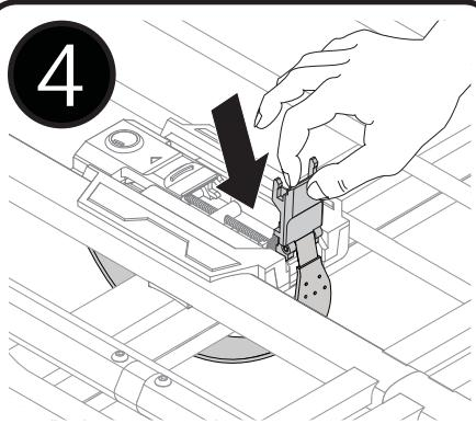
Route the straps under and around the crossbars. With the straps in place under crossbars, hook the tabs back into the detents.
