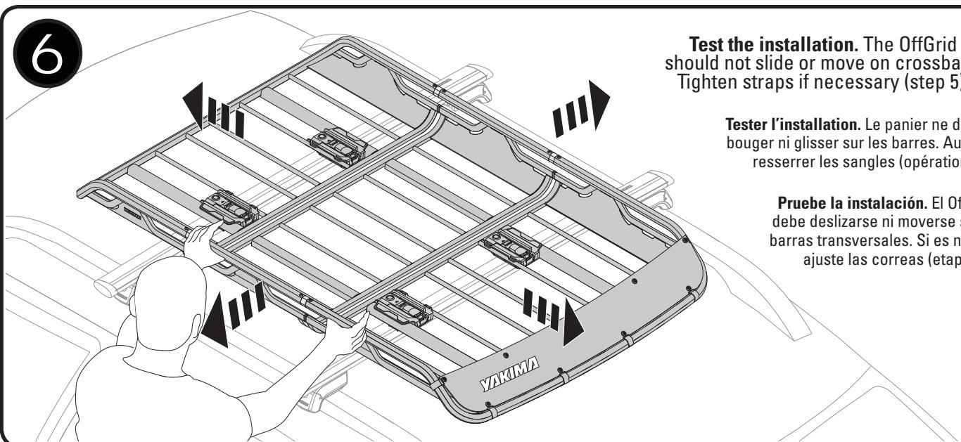
**Test the installation.** The OffGrid should not slide or move on crossbars. Tighten straps if necessary (step 5).
