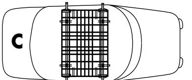
**Be sure the bolts pass through the wire loops on the bottom of the basket.**
