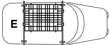
**Be sure the bolts pass through the wire loops on the SIDES of the basket.**
