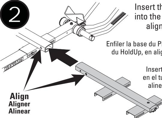
Insert the Plus2 base into the HoldUp tube, aligning holes.
