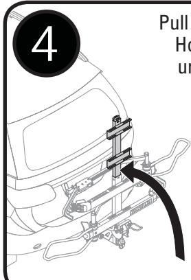
Pull the tilt lever and fold the HoldUp Evo all the way up until it locks into position.
