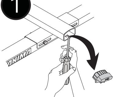
Using a flathead screwdriver remove the end cap from HoldUp EVO.
