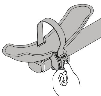
Release wheelstrap by pressing the lever on the buckle.
