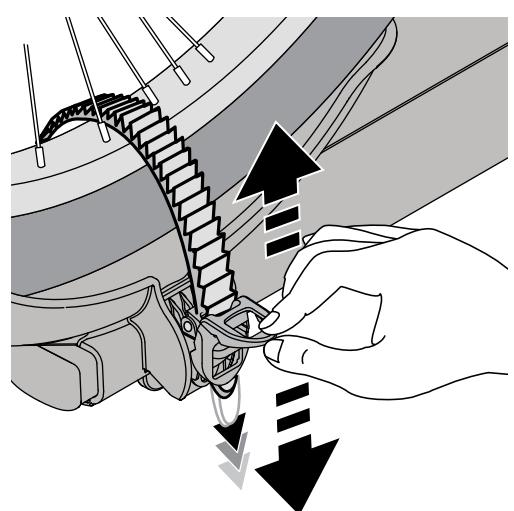
*Move the ratchet tab up and down to tighten the strap.*
