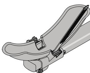
Secure support tube using supplied wrench. Fasten and tighten both sets of bolts, washers, and lock washers.
