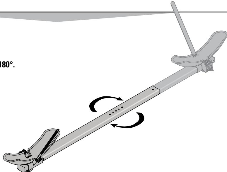
Place rotated support tube back on bracket. Align holes.
