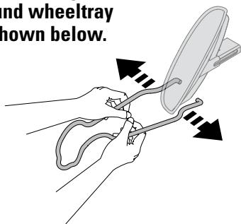
Release letting wire rest in hole, and slot of wheeltray.
