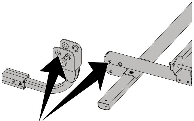
Align holes on tongue assembly with holes on main assembly.
