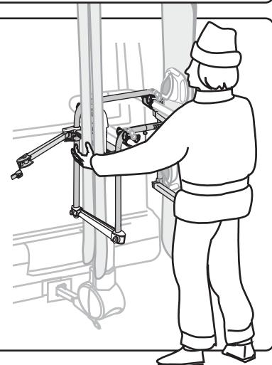
**TO UNLOAD,** unlock and open the cam levers. It is not necessary to loosen the adjustment wheels when unloading.
