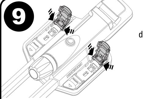
Snap the new levers into their detents and close. Then slide the covers closed.
