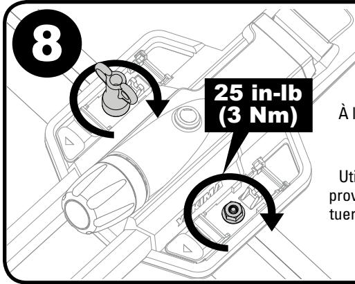
Using the supplied tool fully tighten the nuts.
