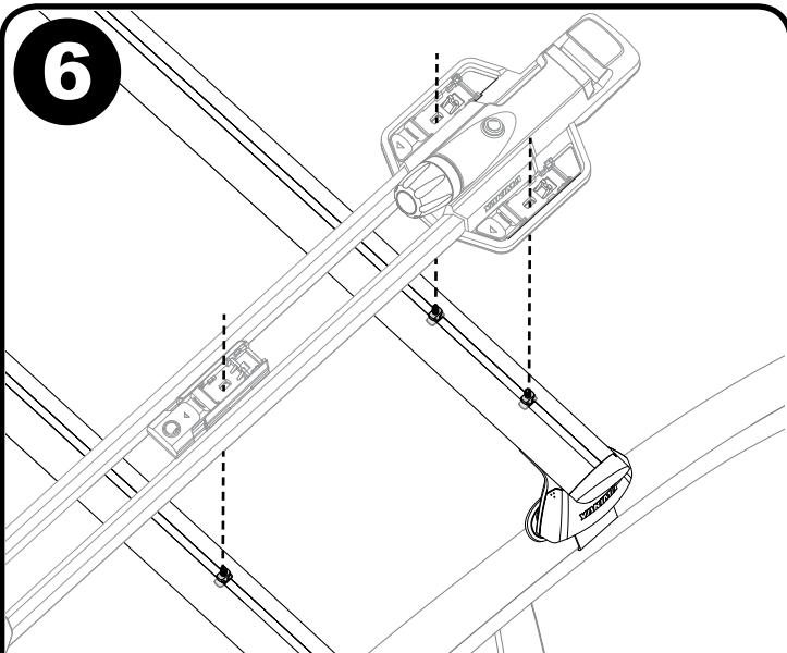
Adjust T-Bolt position as necessary, and carefully lower your carrier onto the T-Bolts.
