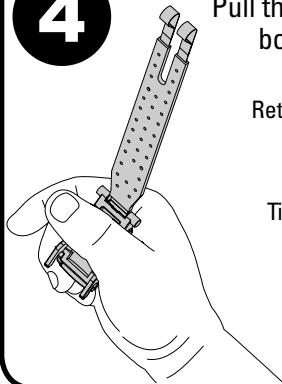
Pull the 3 straps free through bottom of the carrier.
