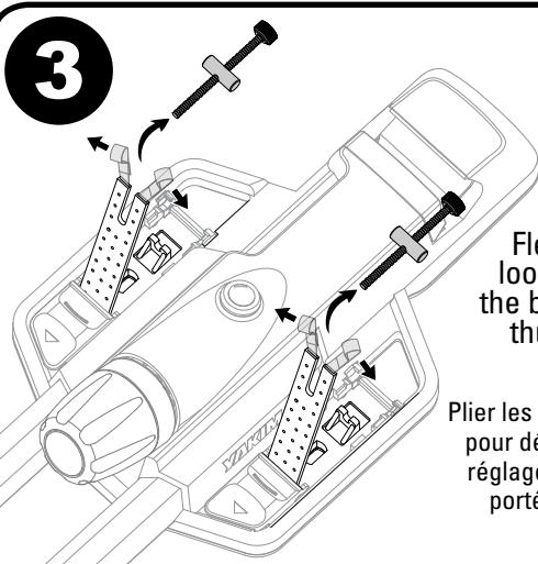
Flex the metal loops to remove the barrel nuts and thumbscrews.
