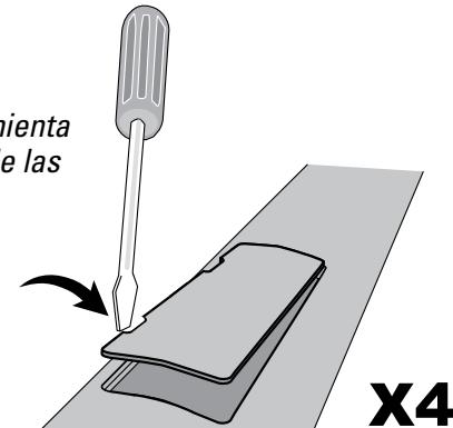
**3 LOCALICE LOS ORIFICIOS DE FÁBRICA.**
