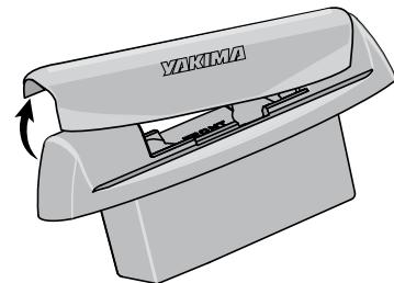
When the racks are not installed, use the covers to keep the bases free of debris.
